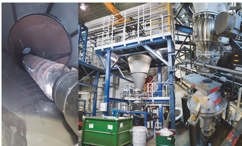
Figure 7. Nauta type vertical cone screw blender for automotive catalysts
