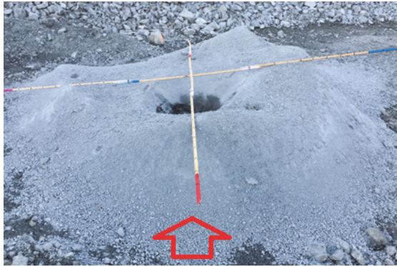
Figure 8. Material around the rotary percussion drilling cone of blast hole (BH01). Note the material size segregation
