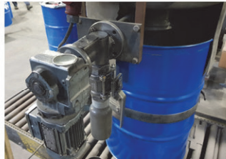
Figure 14. Screw sampler – Coarse fraction within ashes
