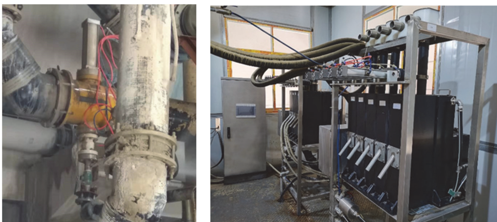
Figure 8. On-line sampler and multiple-channel divider of slurry
