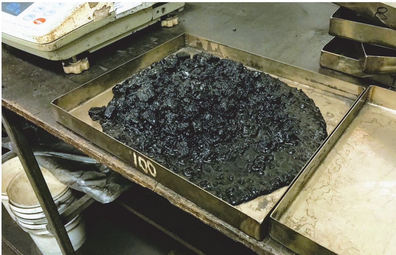
Figure 3. Sample immediately after crushing (during sample preparation), pre-drying was not possible and moisture loss has likely occurred
