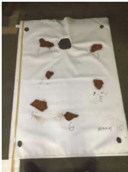
Figures 9 and 10. Samples positioned on filter press clothes for each frame selected for more thorough analyses of the distribution of the Nickel content with HH-XRF.
