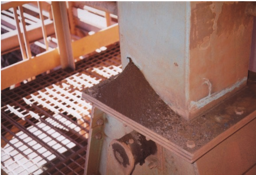
Figure 2. Accessory errors such as sample loss due to holes in chutes need to be eliminated.
