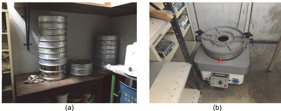
Figure 1: (a) Nested screens for separating ores into correct size fractions, and (b) the mechanical sieve shaker. The distribution of the mass for each of the screened size fractions is shown in Figures 2a and 2b for the Wessels and Mamatwan mines, respectively.
