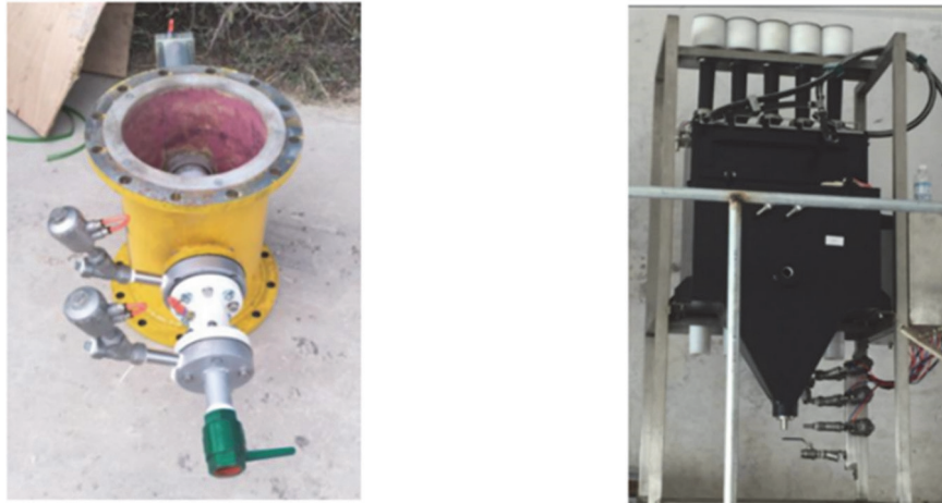
Figure 7. Mobile knife-edge sampler(left) and multiple-channel divider (right)
