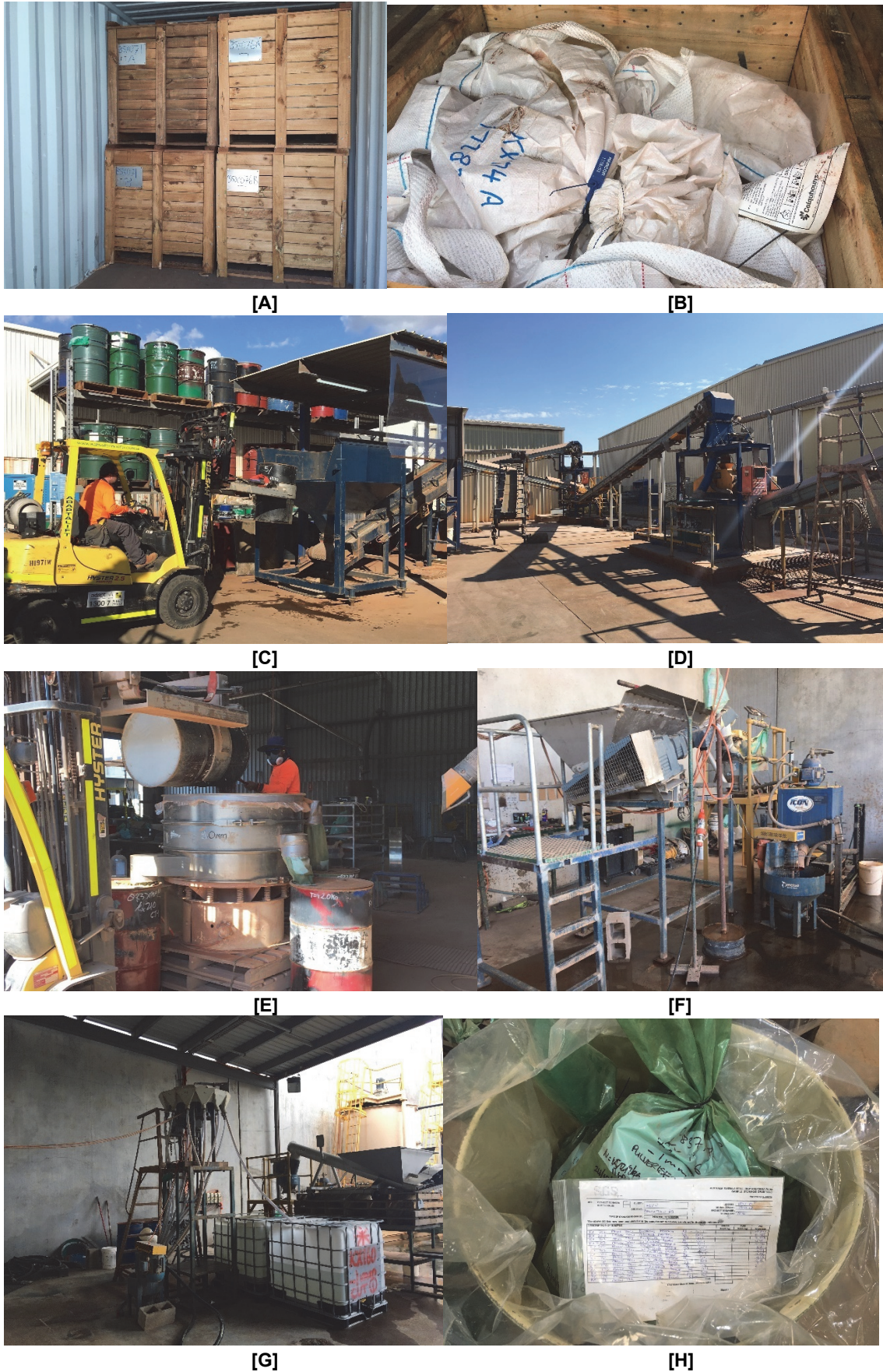
Figure 17. Bulk sample pilot plant: [A] Sealed samples boxes at the laboratory; [B] Tagged bulka bag within transport box; [C] Sample feed to primary crusher; [D] Rolls crusher; [E] Screen process; [F] Gravity concentrator; [G] Gravity tails splitter; [H] Tails samples ready for assay submission.
