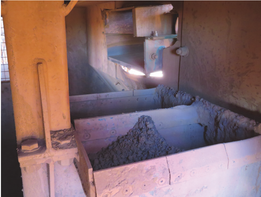
Figure 11. Sample build-up in the secondary cutter apertures.
