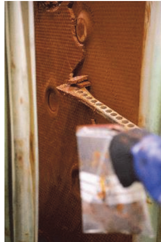
Figure 3. One of the filter press frames with iron sludge. The red framed area marks the most likely reachable region for the manual sample taken by the operators.
