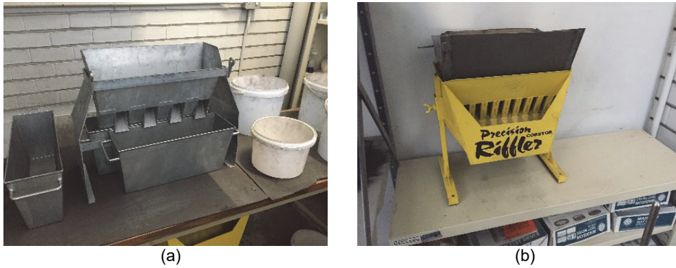
Figure 4: (a) Riffle splitter for coarse materials, >10 mm, and (b) riffle splitter for fine materials, <10 mm Following the splitting process, the samples are bagged (Figure 5a), weighed (Figure 5b), and prepared for dispatch to the analytical laboratories (Figure 5c).
