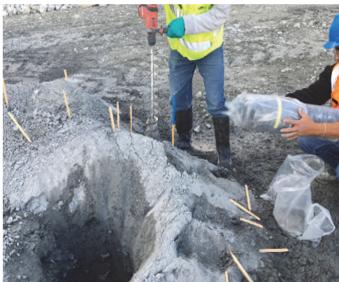
Figure 4. 80-millimeter diameter electric powered, hand-held auger collecting samples perpendicular to the slope of the cone
