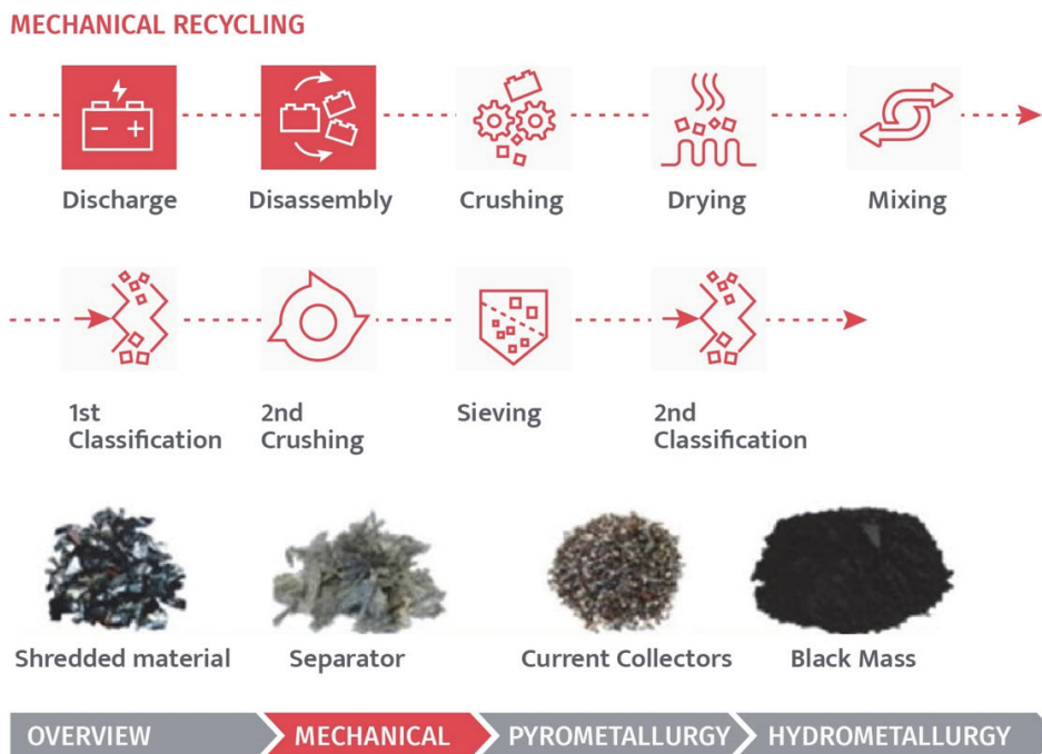
Figure 3. Mechanical stages of LIBs recycling.
