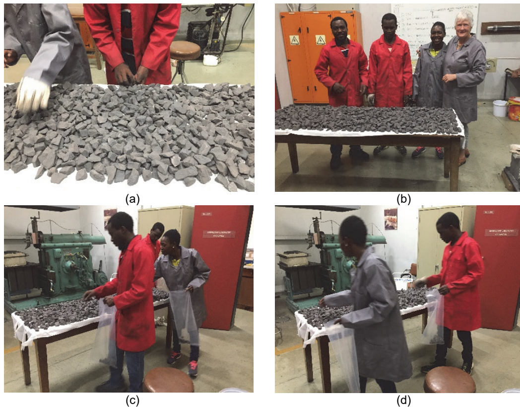
Figure 3: (a) Coarse ore fragments laid on table, (b) the sampling team in preparation for selecting coarse ore fragments at random, (c) as the team moves around the table, they select a given number of fragments at random to achieve the correct sample mass, and (d) the team moves around the table collecting fragments at random
