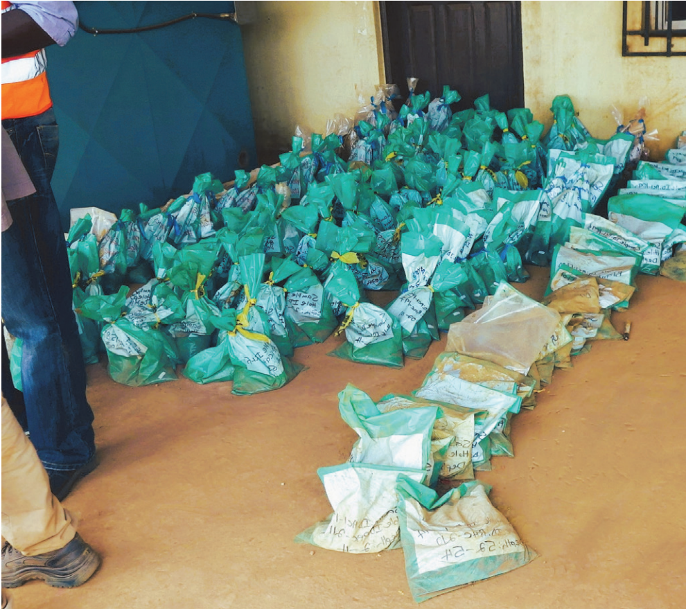
Figure 1. Samples in their non-absorbent air-tight bags awaiting drying soonest after sampling for best integrity
