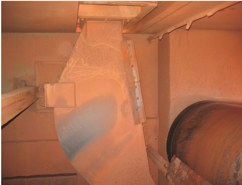
Figure 5. Well-designed primary cutter with a large body for sampling high-capacity streams without reflux from the cutter aperture.
