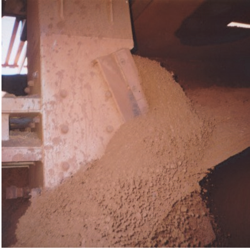
Figure 4. Sample reflux from a poorly designed primary cutter with a narrow body and limited sample capacity.
