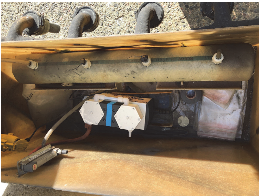
Figure 3. Shows the inside of the box, with the air chamber, flow meter and pump. The wide diameter of the air chamber is large compared to tubes to each sampler, which gives fairly equal airflow through each filter. The flowmeter was calibrated before deployment of the unit.
