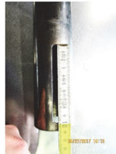
Figure 14. Screw sampler – Coarse fraction within ashes
