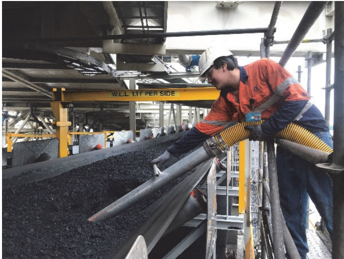
Figure 3. Belt sampling using the vacuum system.
