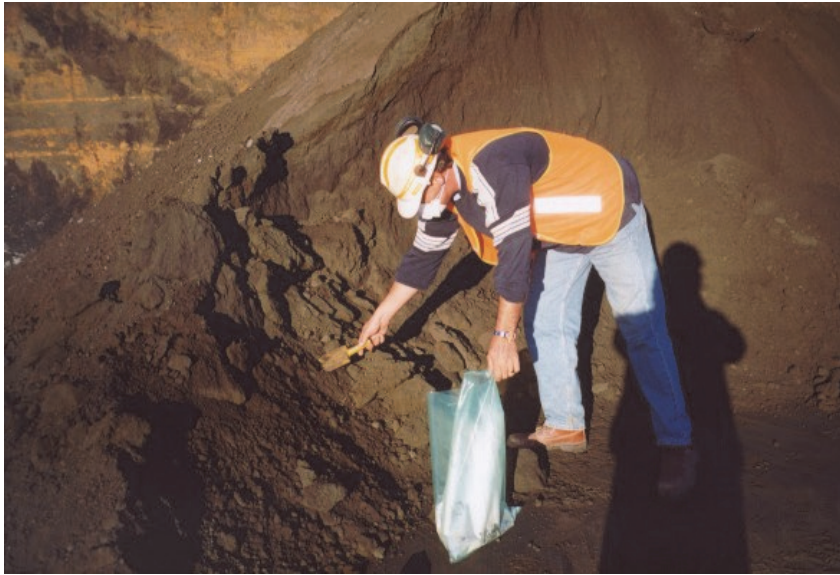
Figure 1. Sampling from the side of a stockpile is problematic and will not provide a representative sample.
