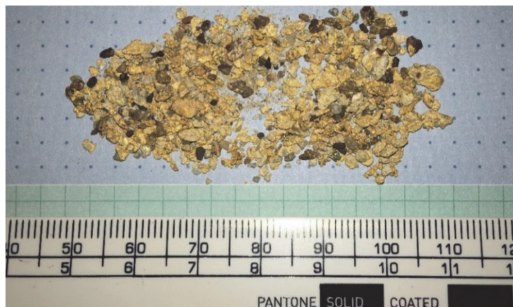
Figure 10. Very coarse gold fraction from a trial mining parcel collected/processed in 2017 yielding a head grade of 1.9 g/t Au.
