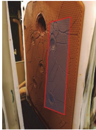
Figure 3. One of the filter press frames with iron sludge. The red framed area marks the most likely reachable region for the manual sample taken by the operators.
