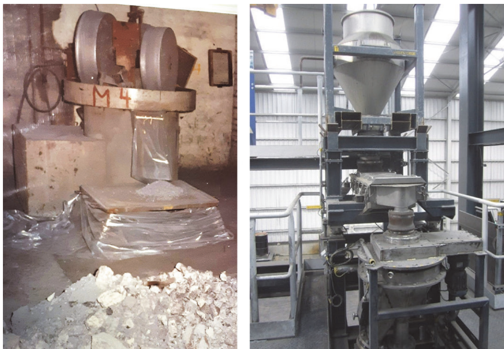
Figure 6. Pan Mill – Before: Manual screening followed by coning a quartering – After: automated sampling after milling with rotary tube divider
