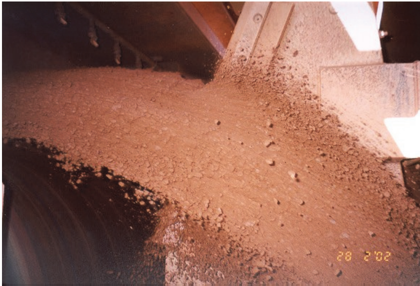
Figure 6. Sampling a high-capacity stream with a well dimensioned primary cutter displaying no sample reflux.
