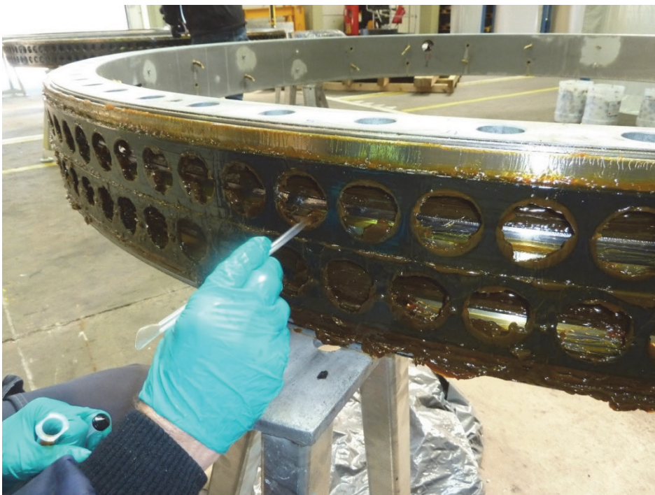
Figure 4. Representative reference grease sampling (TOS) from a dismantled 3.6 MW blade bearing. Increments from every second ball support hole were taken for the 3-D heterogeneity characterization of the grease in the complete 360 degree active zone in the space between the raceways, furthering a reference analogue to "stopped belt" sampling.
