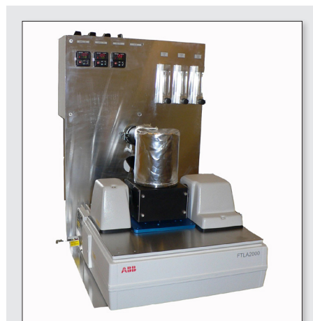
Benchtop gas analytical setup: a modified IR instrument equipped with the necessary pre-analysis hardware. Photo credit: Q-Interline.
