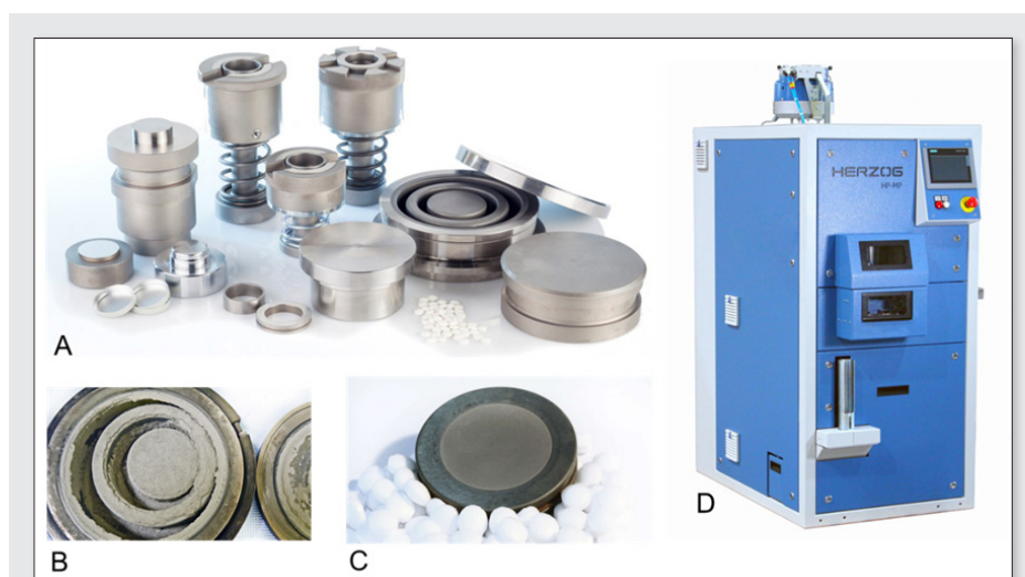
Figure 1. Examples of sample preparation equipment for pressed pellet preparation used in automated XRF analysis. A: Various grinding and pressing accessories for manual sample preparation setup. B: Grinding vessel with sample material. C: Finished pressed pellet suitable for XRF analysis. D: Mill and press combination (HP-MP) used in automatic sample preparation for XRF analysis.
