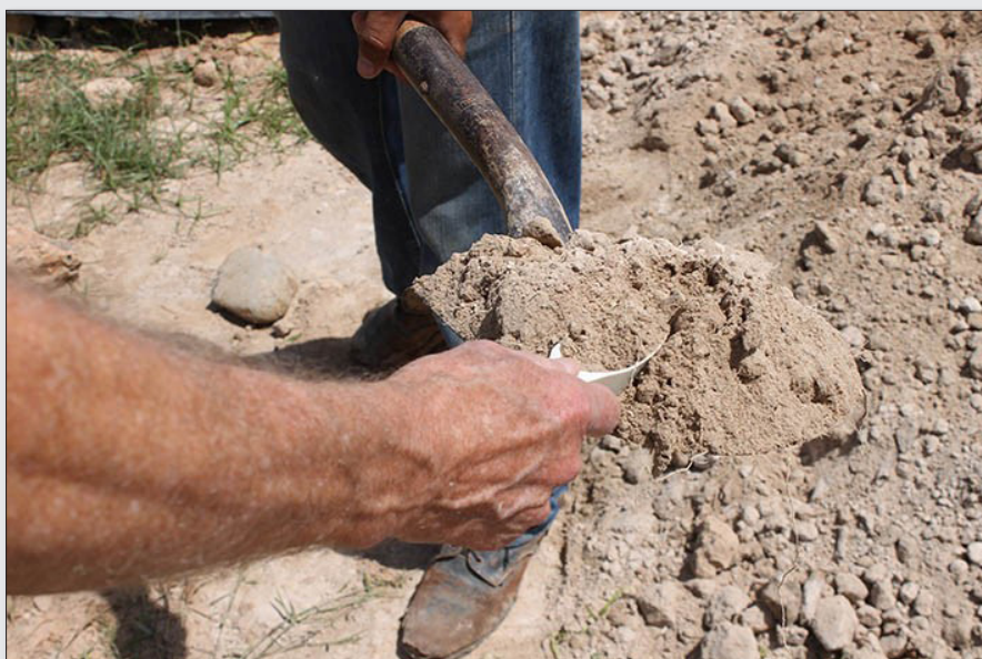
Figure 4. Incremental sampling from each shovel used to transport all original lots, see Figure 3.
