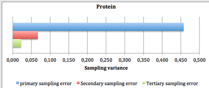
Figure 3. Typical example of comparison of sampling variances from different sampling stages. Dominance of primary sampling variance over secondary and tertiary sampling variance is the typical case.
