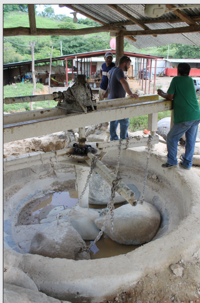
Figure 2. Low tech milling (rastra) with mercury addition (Nicaragua). The boulders mill around slowly for a couple of hours. When milling is complete, the cavity is cleaned of milled ore and mercury amalgamated with gold. The flour floats away.
