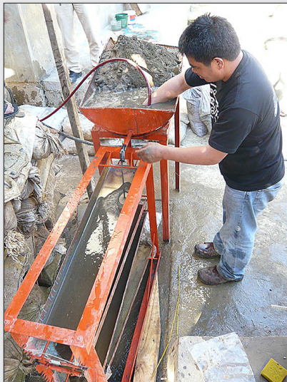
Figure 6. Prototype of “Peter Plates” in action (Philippines). Tailing slurry from the tub is passed over the plates in succession.
