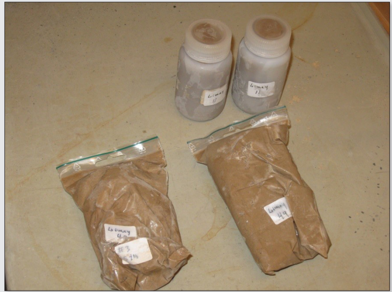
Figure 6. Two types of slurry sample containers as received from Nicaragua, plastic bottles and bags. The photo shows the frozen versions after 24 h in a freezer at –16°C, ready for sub-sampling, see Figures 7–8.
