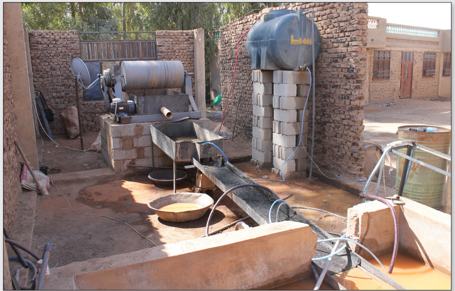
Figure 1. Efficient artisanal processing plant (Sudan) with mill and gravitational processing of pulverised gold ore. The ore is milled in the drum in the background, after which the fine-grained ore is passed through a system of sluices, which concentrates the heavy minerals, including gold.
