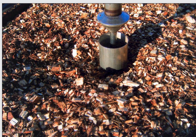
Figure 3. Typical wood shard bio-fuel at a power plant intake. At this plant, routine primary sampling (for moisture determination), takes place following fully TOS-compliant procedures, see Reference 4 for details. An incremental primary increment sampler is shown (centre) just before being inserted into the lot (truckload); the sampler is closed when inserted. Three increments are used for composite sampling, i.e. from the top, middle and bottom level, respectively, with random sampling location in the X-Y plane.
