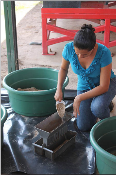
Figure 5. Loading the project riffle splitter (kindly provided by GEUS). Sub-sampling is made effective by the fact that the sample to be split does not need to be split all in one, but can be subjected to riffle-splitting in an intermittent loading process. 7
