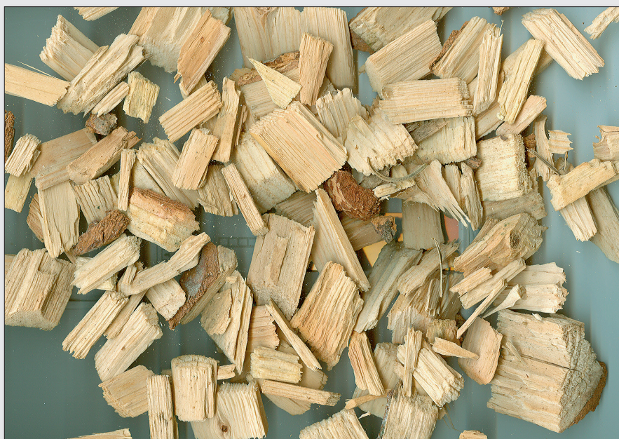
Figure 1. Air dried wood chips used in the original study. Largest shards are approximately 1 inch (3 cm) in length. Although seemingly of uniform composition, the fuel actually consists of a mix of white fir and ponderosa pine. Grab-sampling of the pristine material will obviously give rise to severe sampling errors (FSE + GSE) if not guided by proper TOS-compliant principles, possibly aggravated by using significantly too small sample masses.
