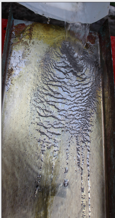
Figure 9. Large amount of mercury captured on Peter Plate (Nicaragua). The plate is about 20 cm wide.
