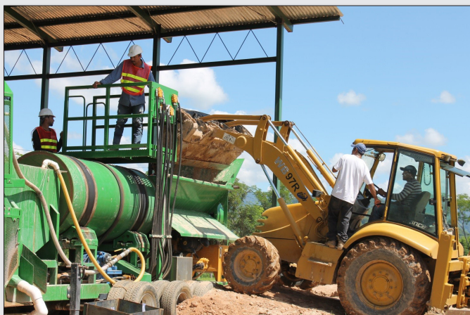
Figure 2. First stage in the SSGM tailing reclaiming process feasibility project, initial particle size screening.
