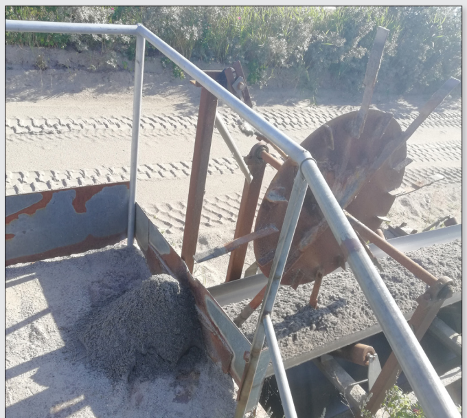
Figure 3. A-ha, the full picture—a two-step sampling solution. Sub-sampling of the primary “sample cone” is also needed (Photo: the Editor).
