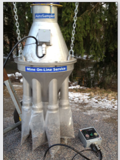
Figure 8. Top: Drillsampler™ from Harrison Cooper for automatic blast hole sampling installed underneath the drill deck (reproduced from Reference 2 with permission). Bottom: the Finnish "Autosampler" system with Softcore™ sample socks attached (reproduced from Reference 24 with permission).
