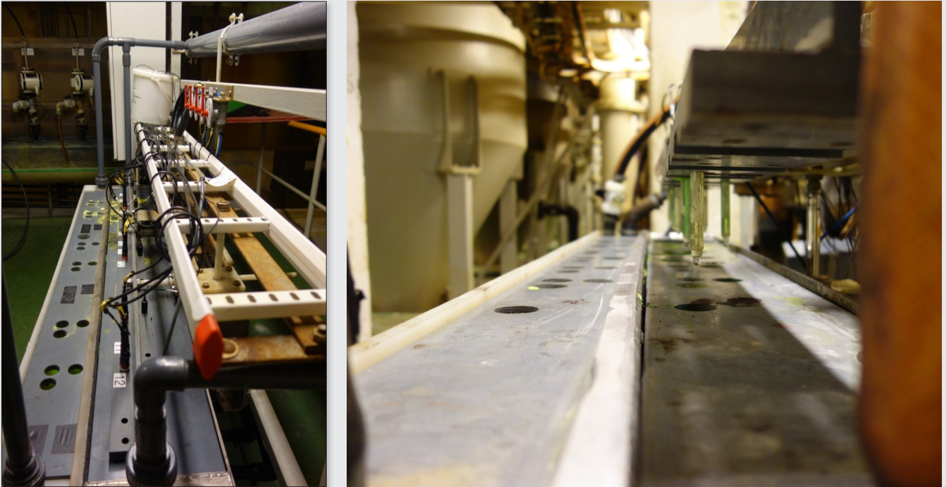
Figure 4. a: Sampling station for pH measurement; b: lifted pH electrodes during the cleaning cycle.
