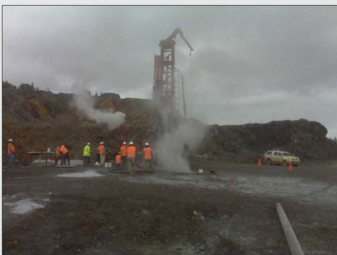
Figure 9. Left: drilling operations using a conventional cyclone and three-tiered splitter system. Right: drilling operations using the PGX1350R sampling system. Reproduced from Reference 14 with permission.
