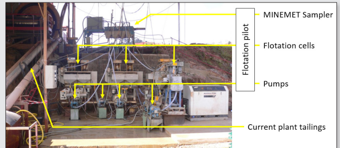
Figure 8. Overview of flotation pilot plant in French Guyana.
