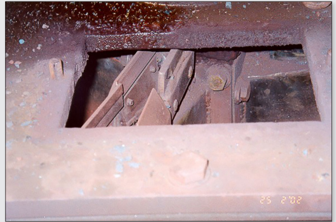
Figure 7. Vezin cutter aperture that is no longer radial due to poor maintenance.
