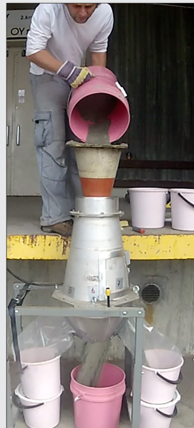
Figure 9. Testing the Autosampler by pouring drill cuttings through it. Two samples are collected in buckets on opposite sides and the reject in the centre.
