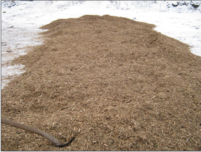
Figure 7. The composite secondary sample lot flattened to a maximum height of 50cm. 50 increments were taken at randomly selected locations and depths (using a shovel), making up the final composite sample of 10kg.
