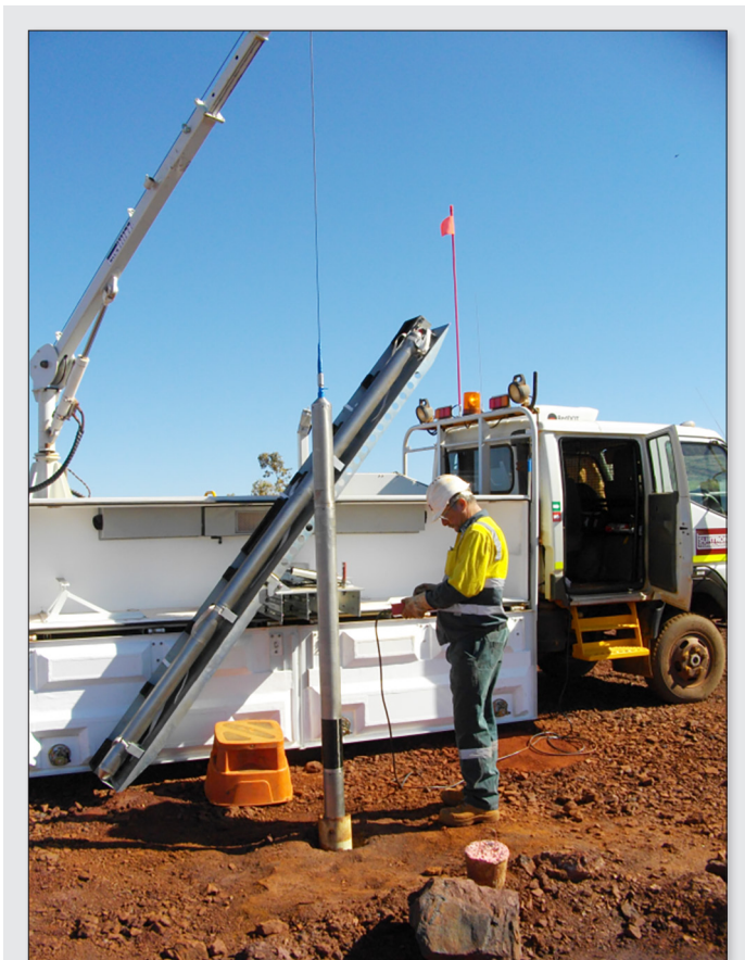
Figure 11. Equipped logging vehicle and FG100 handling
