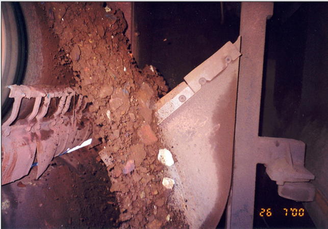
Figure 9. Belt scraper on a head pulley. The primary cutter needs to be moved closer to the head pulley or the cutter aperture extended to intersect all the belt scrapings.
