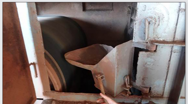
Figure 4. Example of a poorly designed sample cutter that does not traverse the full ore stream.
