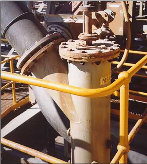
Figure 5. Pressure pipe samplers do not extract a full cross-section of the slurry stream so the samples collected can never be representative.
