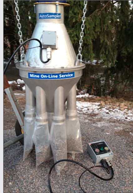
Figure 8. Autosampler system with Softcore™ sample socks attached.
