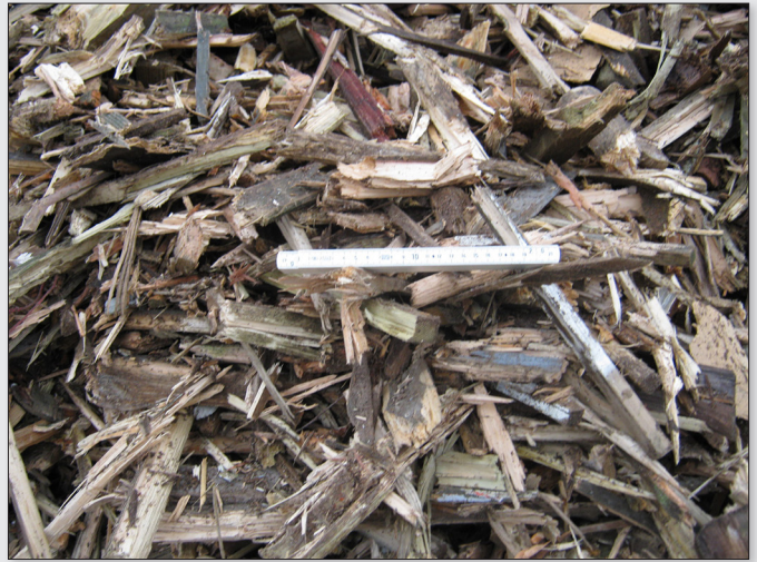
Figure 5. (a) The accumulated primary sample lot (approx. 20 m 3 ). (b) Particle size distribution after primary shredding at step 1 (see Figure 3). A 20 cm folding ruler for scale.
