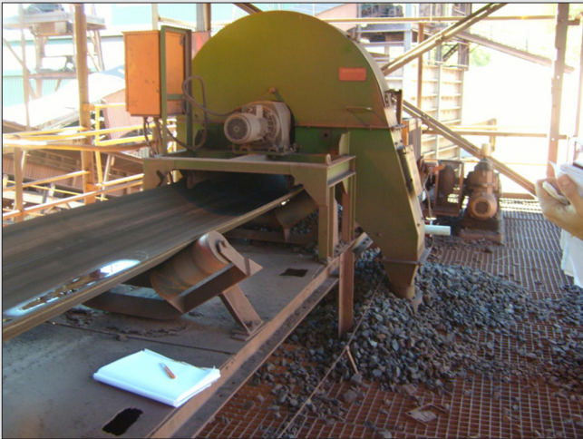
Figure 13. Typical fully enclosed cross-belt sampler installation. While 'hidden' from view, the very poor sampling performance with respect to extraction of a complete cross-section of the stream remains.
