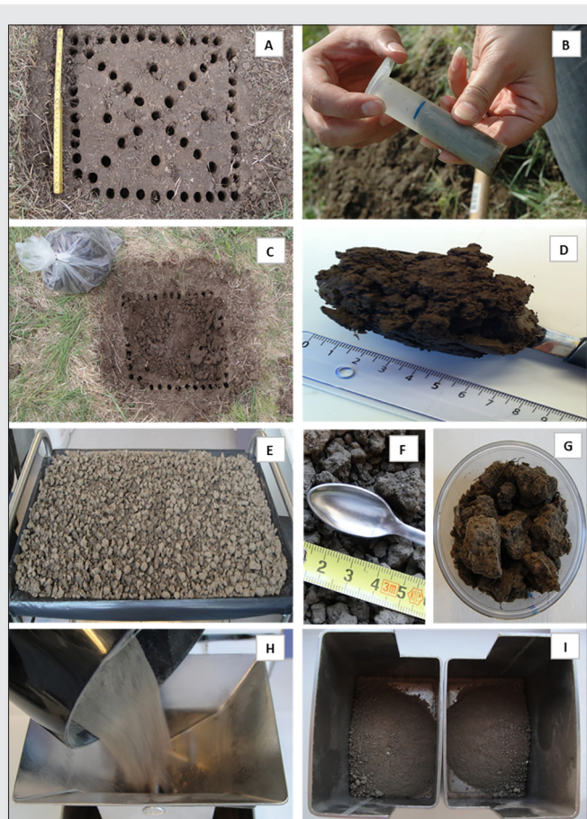
Figure 3. Laboratory mass reduction for clayey soil samples, A) "Small scale 2-D experiment" (50 × 50 cm), B) Single syringe sample; C) Primary bulk grab sample, D) Single grab sub-sample taken from C); E) Remaining bulk sample laid out for composite sub-sampling, F) Increment size, G) Single composite sample (15 increments); H) Single sample after grinding, entering a bespoke laboratory splitter. Identical procedures were applied to all samples in this study. I) Two sub-samples obtain after splitting.
