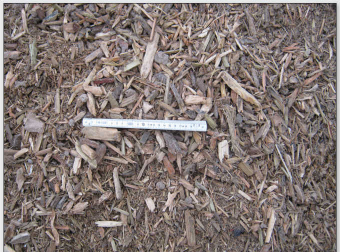
Figure 6. (a) Extraction of increment at step 2 (size reduction to a particle size below 5-10 cm). (b) Particle size after size reduction step 2. A 20 cm ruler for scale.
