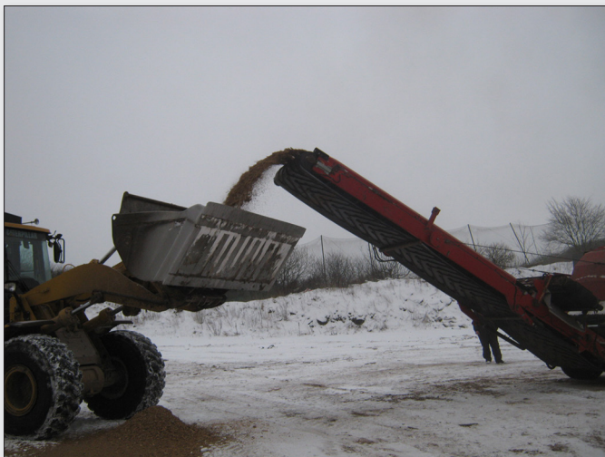
Figure 6. (a) Extraction of increment at step 2 (size reduction to a particle size below 5-10 cm). (b) Particle size after size reduction step 2. A 20 cm ruler for scale.
