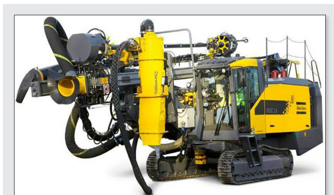
Figure 1. RC ROC L8 drilling rig with automatic sampling system.
