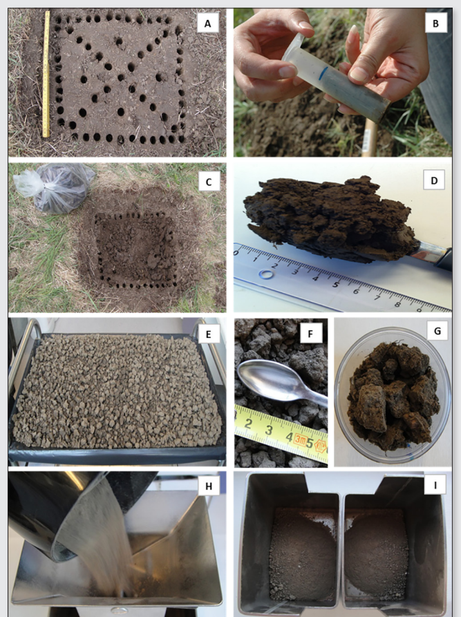
Figure 3. Laboratory mass reduction for clayey soil samples, A) "Small scale 2-D experiment" (50 × 50 cm), B) Single syringe sample; C) Primary bulk grab sample, D) Single grab sub-sample taken from C); E) Remaining bulk sample laid out for composite sub-sampling, F) Increment size, G) Single composite sample (15 increments); H) Single sample after grinding, entering a bespoke laboratory splitter. Identical procedures were applied to all samples in this study. I) Two sub-samples obtain after splitting.
