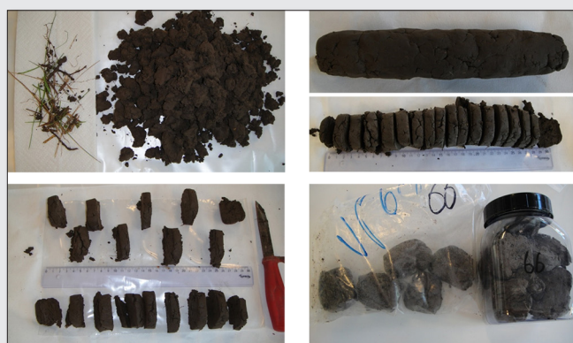
Figure 4: Fresh soil mass-reduction steps for clayey soil. A procedure, identical to riffle splitting, was developed for sub-sampling in the laboratory for this type of mildly sticky, non-flowing material.
