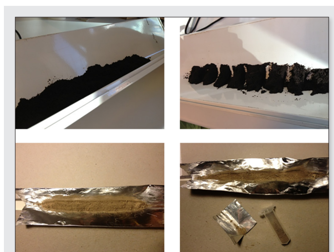
Figure 5. Manual 'riffle-splitting' simulation for representative sub-sampling in the laboratory. This technique is also known as bed-blending, scaled-down and adapted to both dried, but still cohesive primary sandy soil samples (top) as well as to fine-crushed, dried powder (bottom). This procedure can be described as 'linear bed blending/transverse thin-slice reclaiming'.
