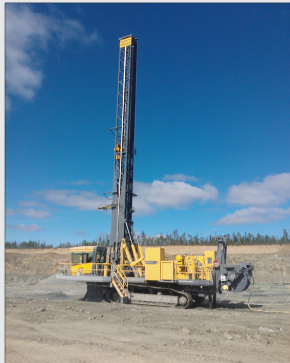
Figure 4. Atlas Copco Pit Viper 271 Rotary drill at Kaunisvaara iron ore mine
