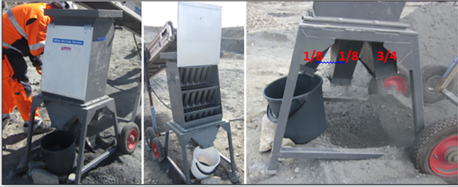
Figure 5. A Metzke model MFS 3T32 3C 3-tier splitter was used at the end of the conveyor belt to split collected drill cuttings at ratios 1/8 , 1/8, 3/4, as shown above right.
