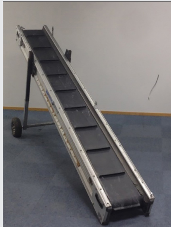
Figure 3. Primary sampling belt conveyor used in this study. Conveyor width was 400mm and length 3 meters.
