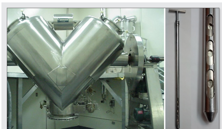
Figure 2. Sampling thieves are used extensively to extract single samples from blenders with various fixed geometrical schemes. 13 Left: large V-blender used in pharmaceutical industry; right: expanded view of sample thief and die cavity.
