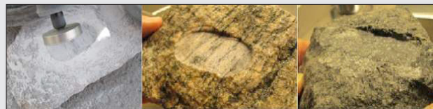
Improved surface hXRF fidelity resulting from application of the newly developed Field Rotary Abrasion Tool (FRAT) 2
