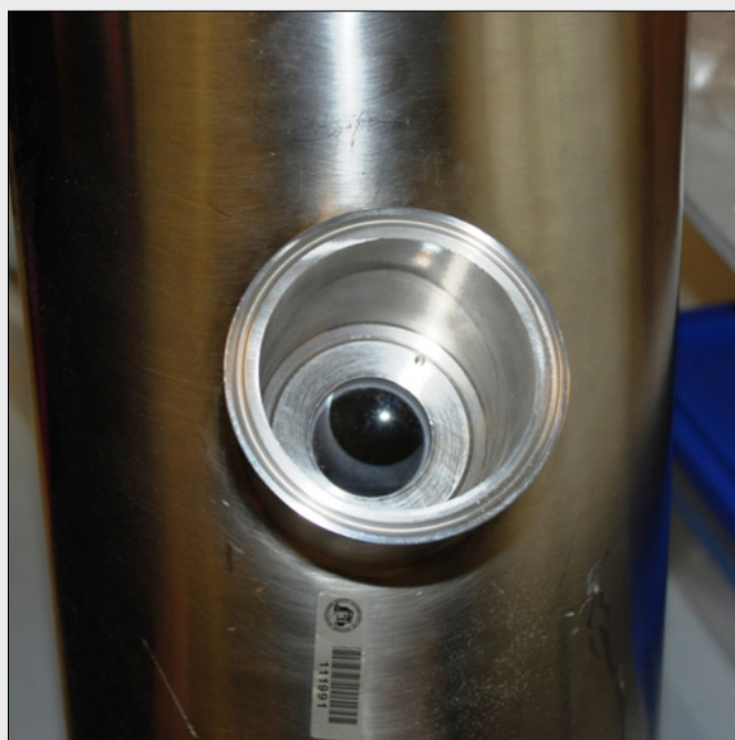
Figure 3. The “no sampling” fallacy in PAT. The NIR spectrometer is optically sampling the powder within the blender through a sapphire window. Left: tumble blender and wireless NIR spectrometer that rotates with the blender. The spectrometer obtains a signal for the material but only to a depth of less than 2 mm below of the window shown on the right. The remaining part of the material is not analysed. The assumption is that the vigorous mixing/blending allows for a meaningful averaging of the signal characterisation of the whole volume. This is a lab-scale system; typically manufacturing tumble blenders are much larger, which introduces ever greater scale-up issues.
