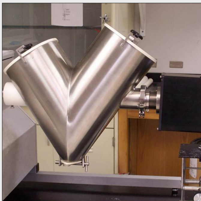
Figure 3. The “no sampling” fallacy in PAT. The NIR spectrometer is optically sampling the powder within the blender through a sapphire window. Left: tumble blender and wireless NIR spectrometer that rotates with the blender. The spectrometer obtains a signal for the material but only to a depth of less than 2 mm below of the window shown on the right. The remaining part of the material is not analysed. The assumption is that the vigorous mixing/blending allows for a meaningful averaging of the signal characterisation of the whole volume. This is a lab-scale system; typically manufacturing tumble blenders are much larger, which introduces ever greater scale-up issues.
