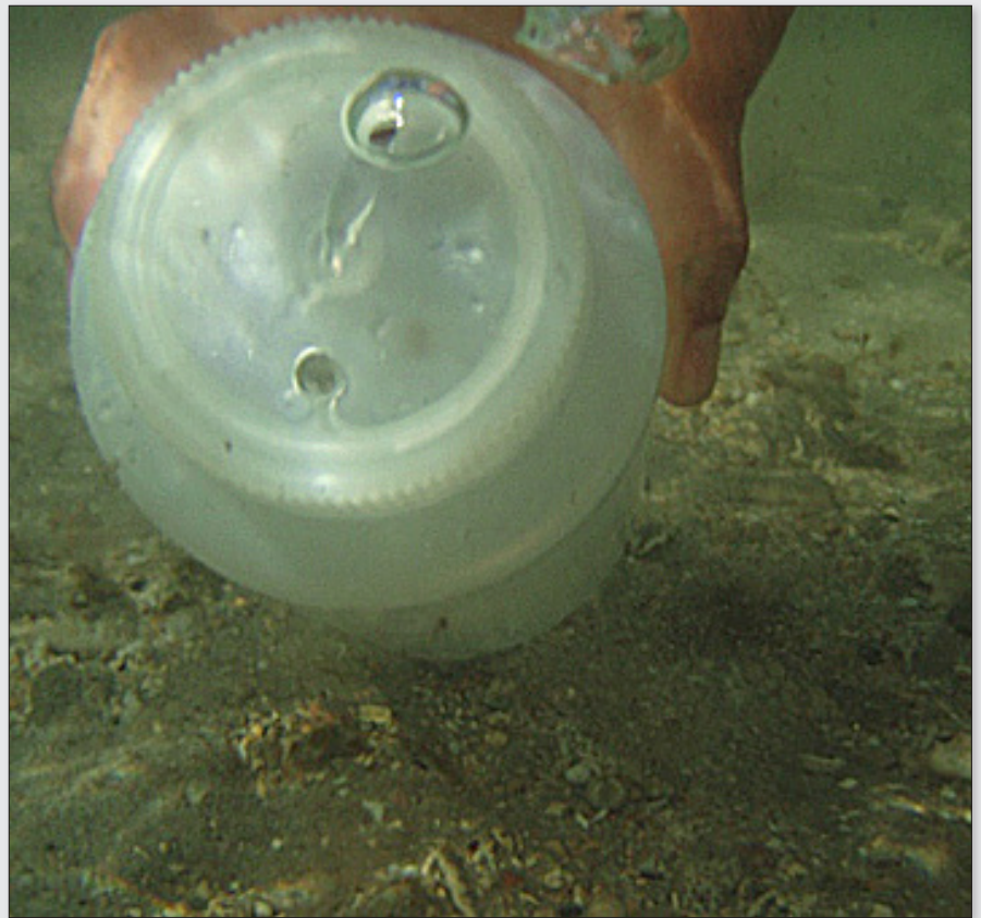
Figure 6. The Aloha Sampler in operation. Note air bubble leaving the upper hole in the aperture cover.
