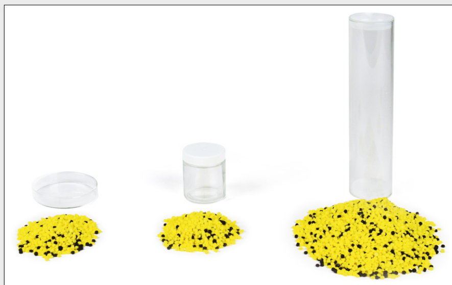
Figure 3. Illustration of the different sample masses typically achieved with the Petri dish (left), rolling bottle (centre) and spiral sampler (right). Typical proportions between the effective analytical masses are 35 g, 50 g and 600 g, respectively. N.B. the analytical NIR sensor system does not interact with the entire mass in the containers.
