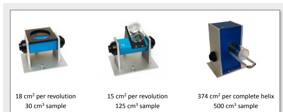
Figure 1. Illustration of the different NIR accessories [Petri sampler (left), bottle sampler (centre) and spiral sampler (right)] which present the sample to the spectrometer in three different ways. The effective scanned areas are also indicated (dependent on method/number of scans) and the maximum sample volume for the respective sample containers.
