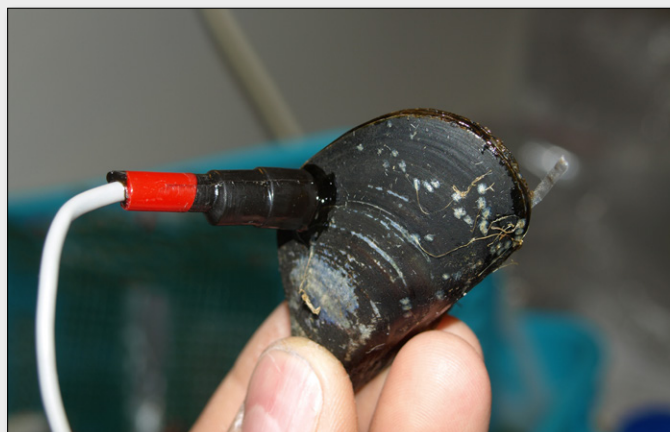
Figure 3. Instrumented bivalves fitted with an infrared sensor for heart rate determination (left), and with added calipers for recording valve gape (opening-closing) characteristics as well (right).
