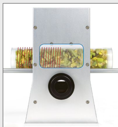
Q-Interline's Spiral Sampler acquires representative data from very heterogeneous samples.
