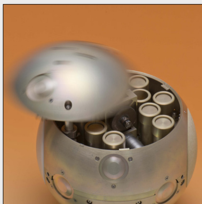
This spherical container has been engineered to house samples to be brought back from Mars. Weighing less than 5 kg, this 23 cm-diameter sphere has been designed to keep Martian samples in pristine condition at a temperature of under -10^{\circ}\text{C} throughout their journey back to Earth. The container hosts 11 sealable receptacles, including one set aside for a sample of martian air. Copyright ESA-Anneke Le Floch
