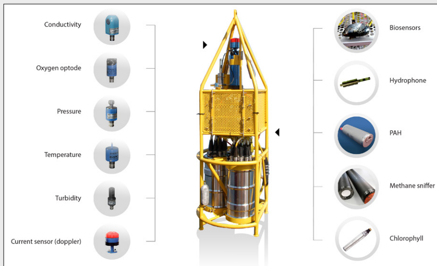
Figure 2. Biota Guard Marine Monitoring System station. The full complement of conventional oceanographic, PAT and the novel biosensors are shown in the side panels. All sensors are integrated in the subsea station (centre). The biosensors are located in the yellow cage (see further in Figure 3).
