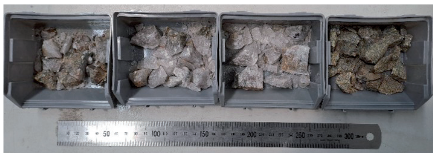
Figure 19: WA Goldfields specimens – post primary fragmentation
