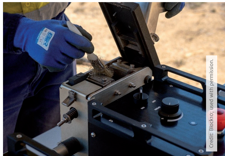
Figure 5: Cleaning the crusher between samples
