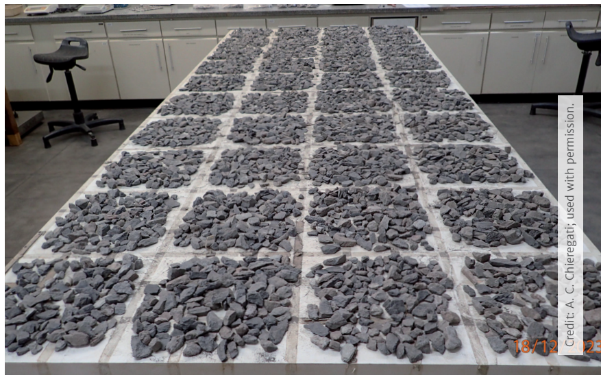
Figure 1: Coarsest size class of the material lot under study retained on the d/2 sieve.
