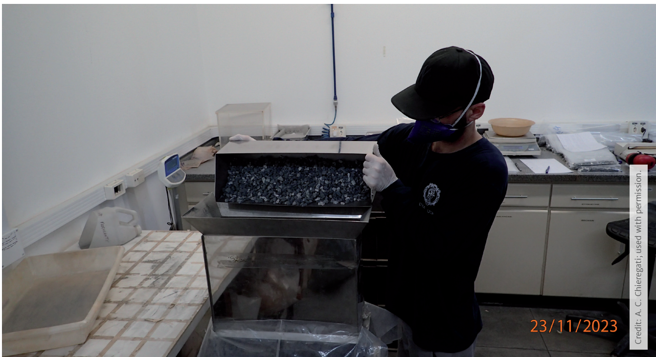
Figure 5: Material of the -1/2'' + 1/4'' size class being riffle split during the STE/SFA procedure.
